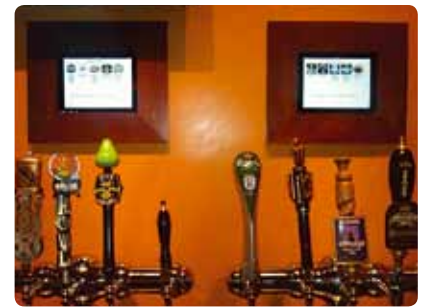
Framed Apple iPads provide customers with information about the beer on that tower, as well as hide Impinj Mini-Guardrail antennas.
